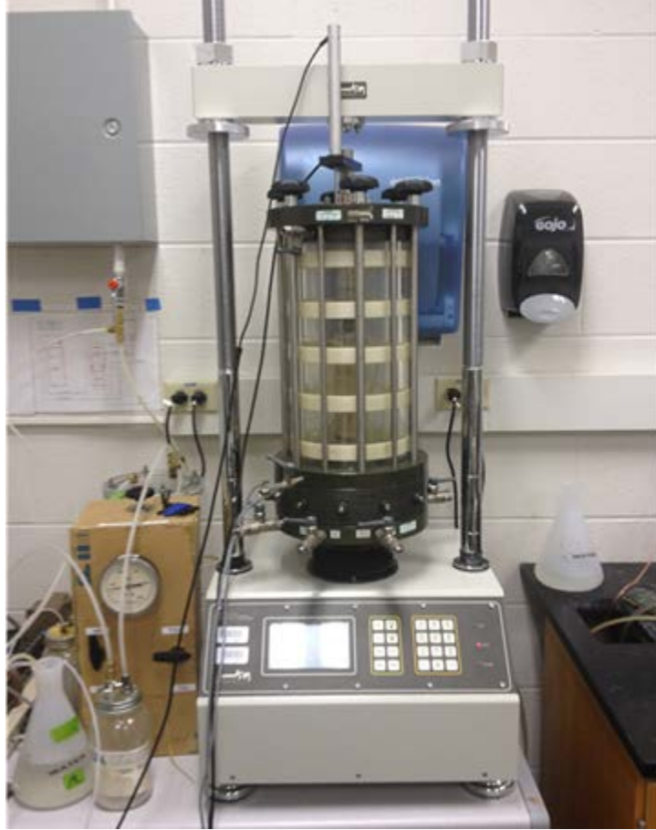
Figure C.22 GDS 50 kN capacity load frame and double walled unsaturated triaxial cell configured for testing.
