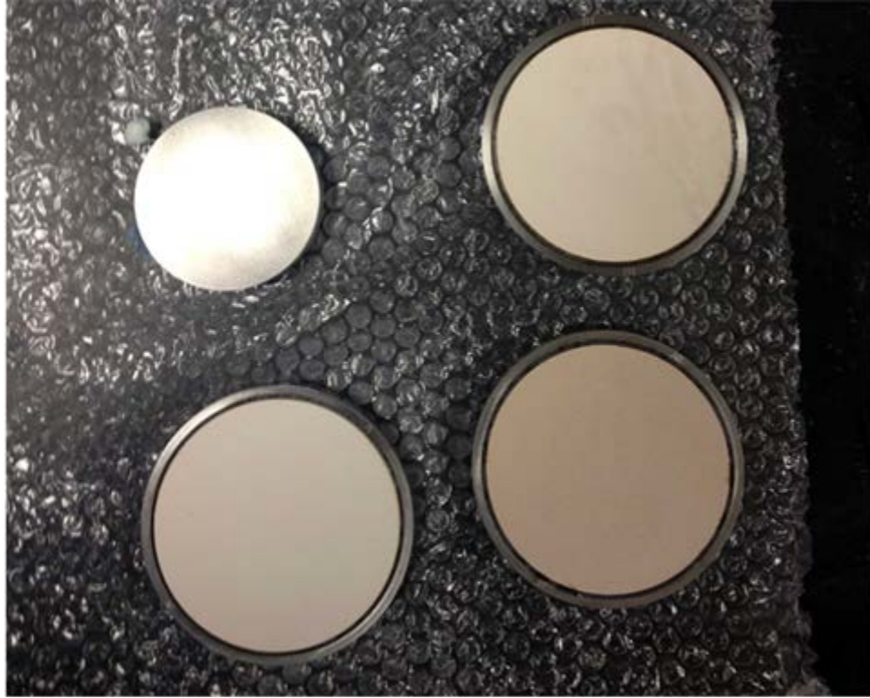
Figure C.4 High air-entry porous ceramic disks for the single cell pressure device shown with and without the stainless steel rings.
