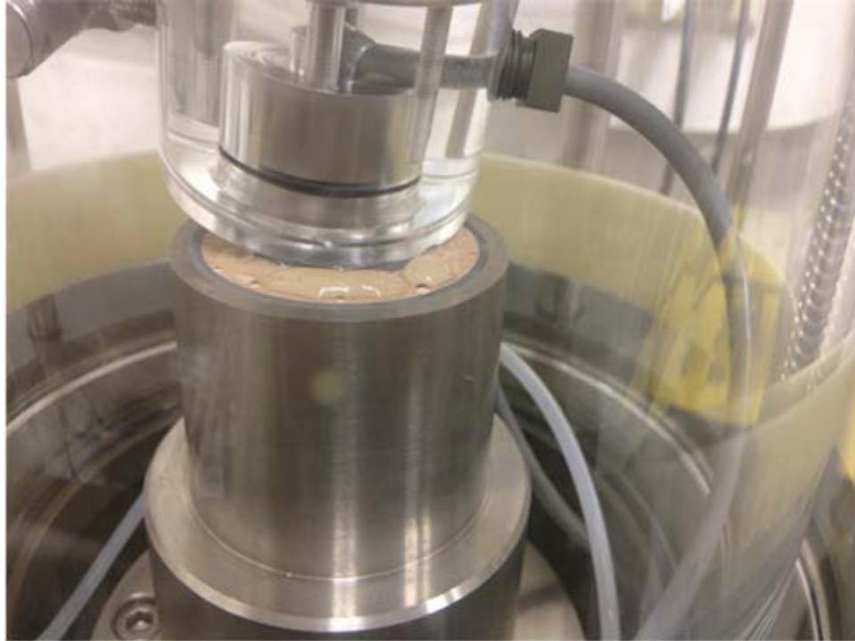
Figure C.29 Water pooling on surface of HAEPD during bottom-up phase of the HAEPD saturation process.
