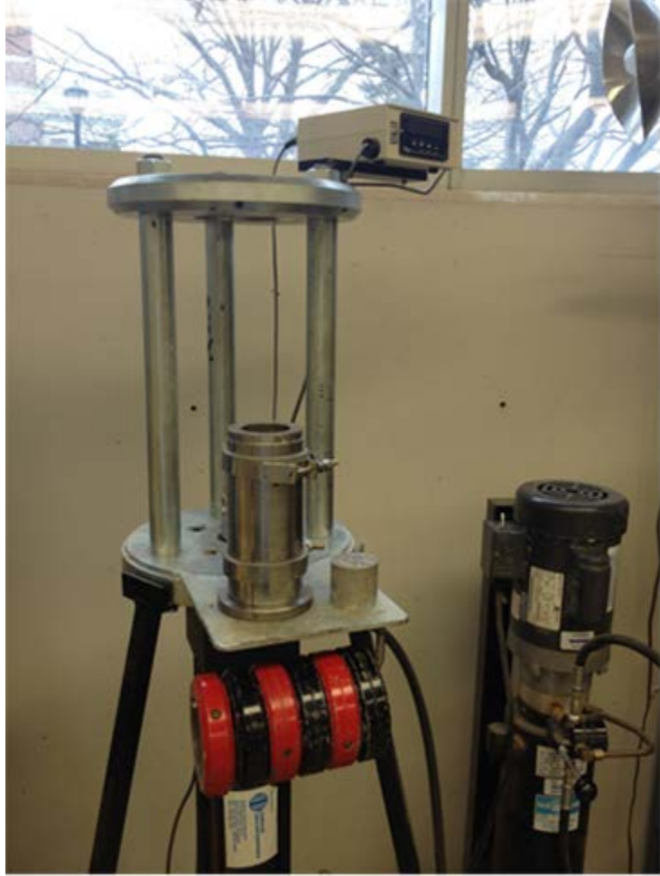
Figure C.27 Unsaturated triaxial specimen 2 inch internal diameter split mold, spacer rings, extruder piston, and the static compactor.
