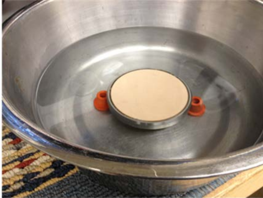
Figure C.14 Initial saturation process of the high air-entry porous ceramic disk elevated with spacers, but completely submerged in de-aired water.
