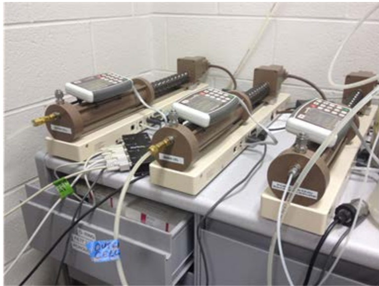
Figure C.23 Standard pressure volume controller v2, STDDPC.
