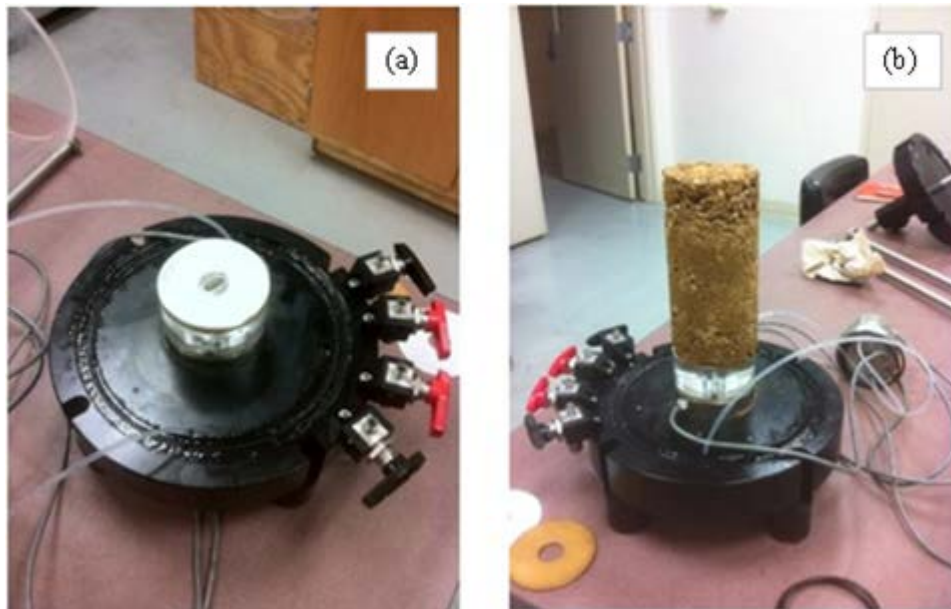
Figure C.20 (a) bottom platen of cell with Bender element and cut-out filter paper; (b) remolded clay sample placed on base pedestal.
