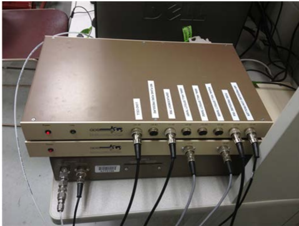
Figure C.26 Control boxes for unsaturated triaxial testing: (bottom) GDS pneumatic pressure controller, GDSPPC; (middle) bender element master control box; and (top) data acquisition 8 channel serial pad.
