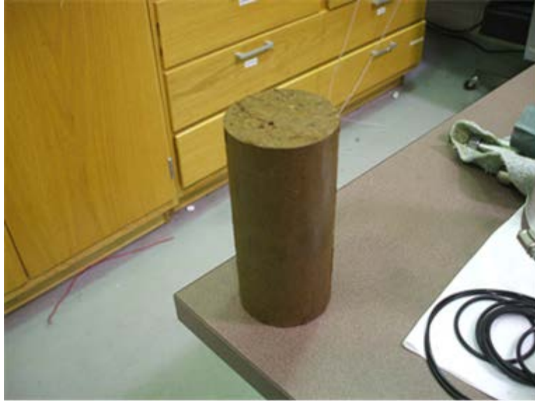
Figure C.19 Typical CIU triaxial soil specimen.
