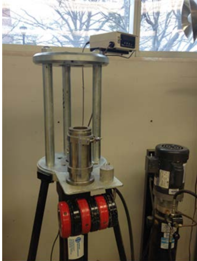
Figure C.7: SWCC specimen molding system consisting of split mold, and the static compactor.
