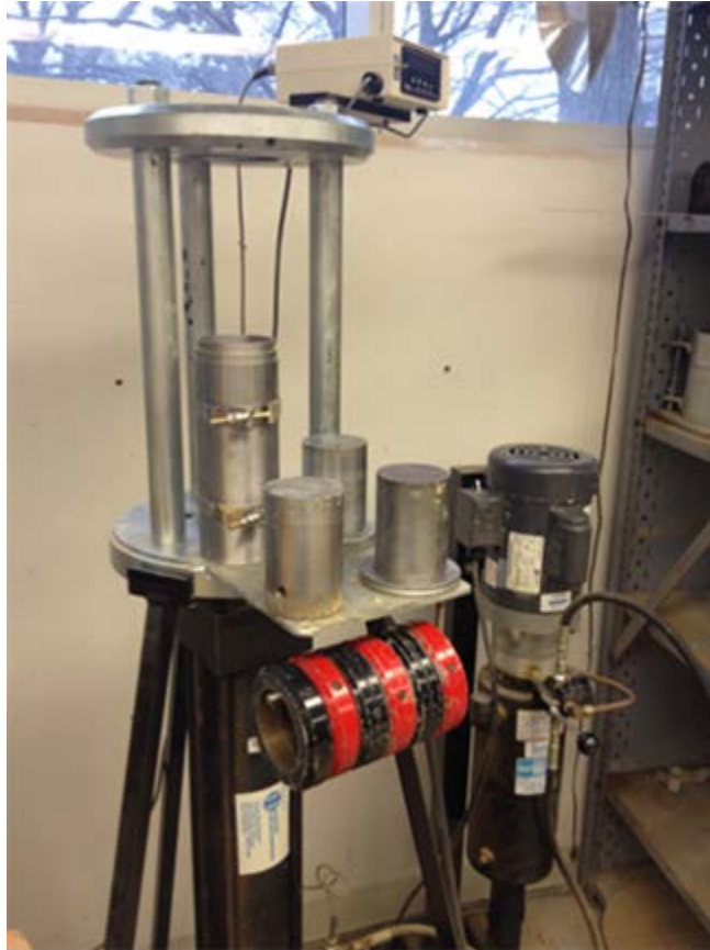
Figure C.17 CIU specimen molding system consisting of split mold, top and bottom pistons, spacer rings, extruder piston, and the static compactor.
