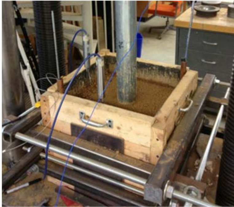
Figure C.40 Shelby tube sampling of the bulk soil.
